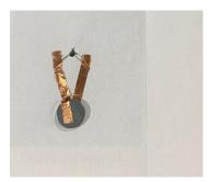
6. Once the LED is lit you can use a piece of clear tape to secure the battery and copper tape to the card to make it a bit more secure.
